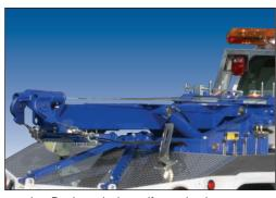
Jerr-Dan's exclusive self-contained recovery boom is hydraulically actuated for raise, lower and extend functions.
